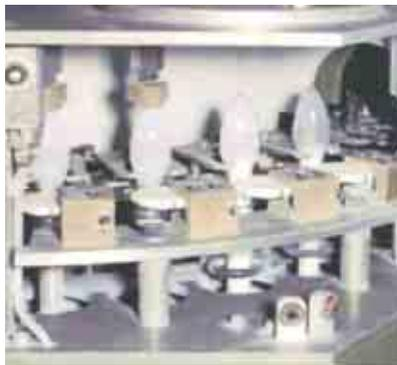
The coating powder is applied by electrostatic process. The colored bulbs are conveyed to the production line. One corona dispersion head is introduced in each bulb.
